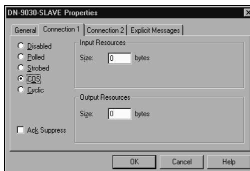
COS I/O Messaging Screen for a Series 90-30 DeviceNet Slave Module
