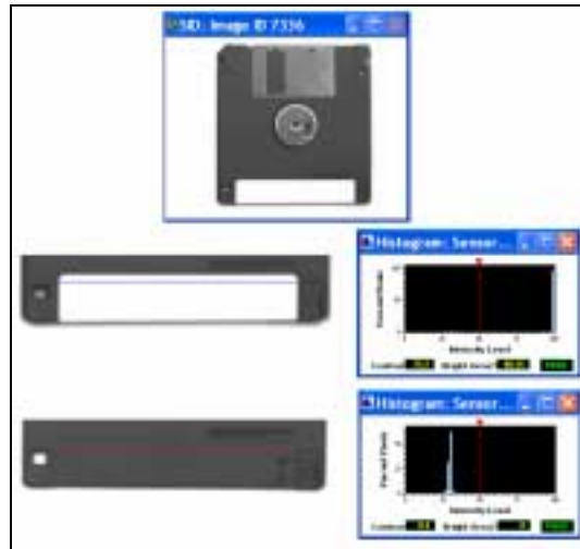
Figure 30: Use of an Intensity SoftSensor to verify the presence and correct position of a label.
