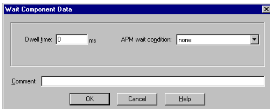
Figure 4-20. Wait Component Data dialog box: Motion Mate APM300 and Motion Mate DSM300
