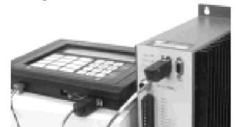
Figure 2.8: OIP Cable Connected to OIP and Controller
