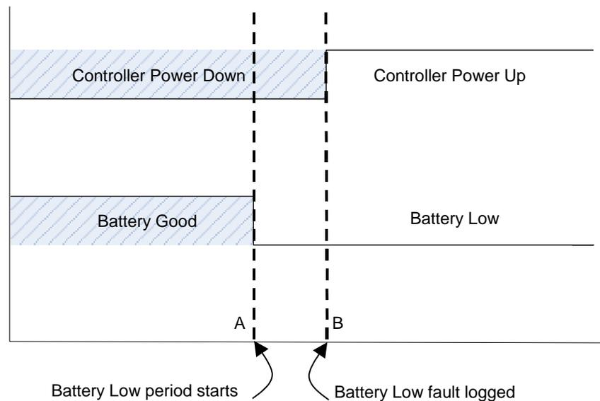
The Battery Low period of 15 days starts at Point A, but the low battery fault is logged only at Point B, once the controller is powered ON. So, the user should make a note that the timestamp of the Low Battery fault may not give the exact start of the 15 days Battery Low period.
