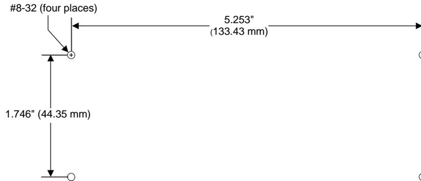
2. Securely attach the Smart Battery Module to the panel mounting surface using four #8-32 x 1/2" flat head machine screws.
