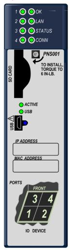
The PACSystems\* RX3i PROFINET Scanner module, IC695PNS001 or PNS001, connects a remote universal RX3i I/O rack of Series 90-30 or RX3i modules to a PROFINET I/O Controller. The PROFINET Scanner scans the modules in its rack, retrieving input data and providing output data, and exchanges that data on the PROFINET I/O LAN at the configured production rate.
